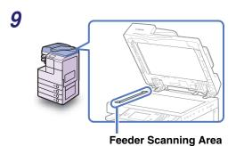
Clean the feeder scanning area (the left side of the platen glass) with a water-moistened cloth. Then, wipe the area with a soft, dry cloth.
